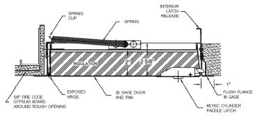
UL, Northbrook, IL - 1-1/2 hour s'B' label for vertical wall installations only. Test file number R-10364. This door may be used in a two hour fire rated wall assembly
